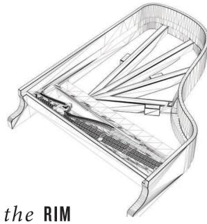
STRAIGHT-GRAINED HARD ROCK MAPLE BENT BY HAND FOR OVER 140 YEARS PATENTED ONE-PIECE CONTINUOUS BENT RIM STATE-OF-THE-ART CONDITIONING
